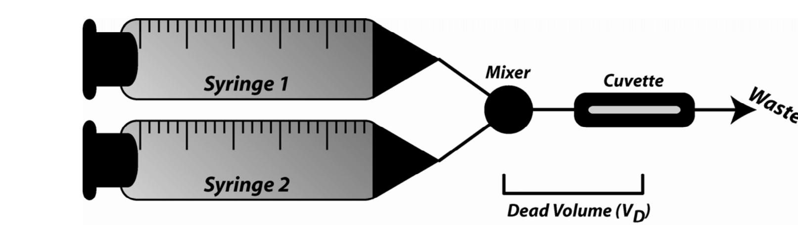
Rapid kinetic experiment was performed at 25°C on the uSFM-20 (Biologic, France) stopped-flow instrument. The mixing volume was 120  $\mu$ L with sampling period at 200 us and 5 ms.
